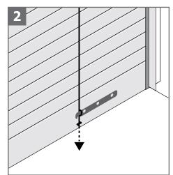
Remove the traction rope from the suspension and pull the rope
