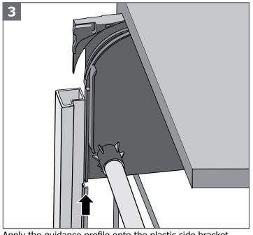
Apply the guidance profile onto the plastic side bracket
