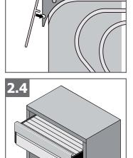
Clips the cover onto the plastic side parts of the unit
