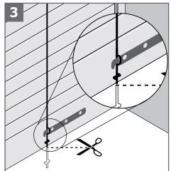
Tie a new knot in the rope and fit it around the suspension
